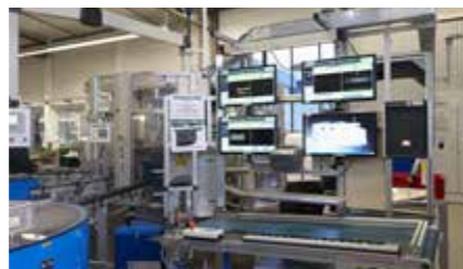
Plug output conveyor and image processing
