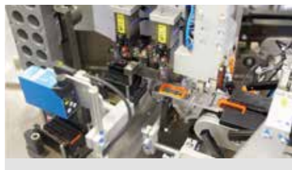
Inserting the radial seal into the contact carrier top
