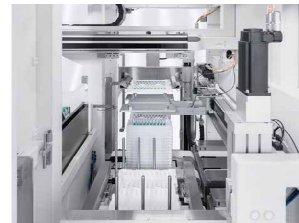
Consistently reliable tray separation, even when flimsy disposable trays are used
