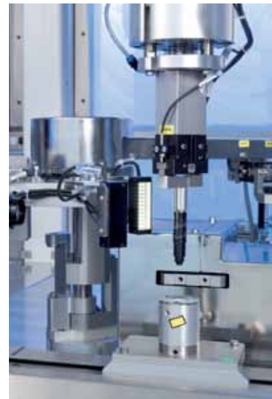
Testing and inserting the dial
