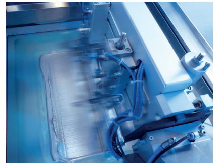
Adhesive application via screen printing
