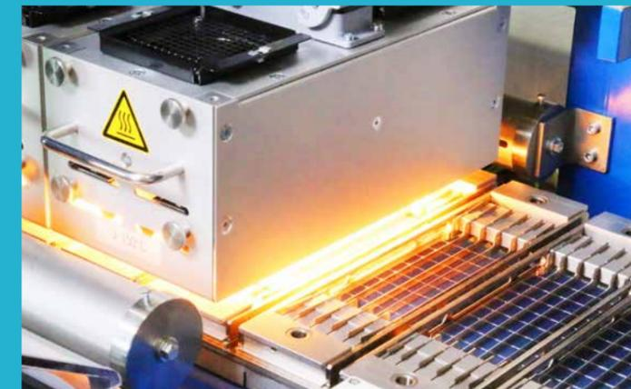
Closed loop IR light soldering process
